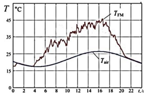
Fig. 7. Heating graph of the PV module surface
