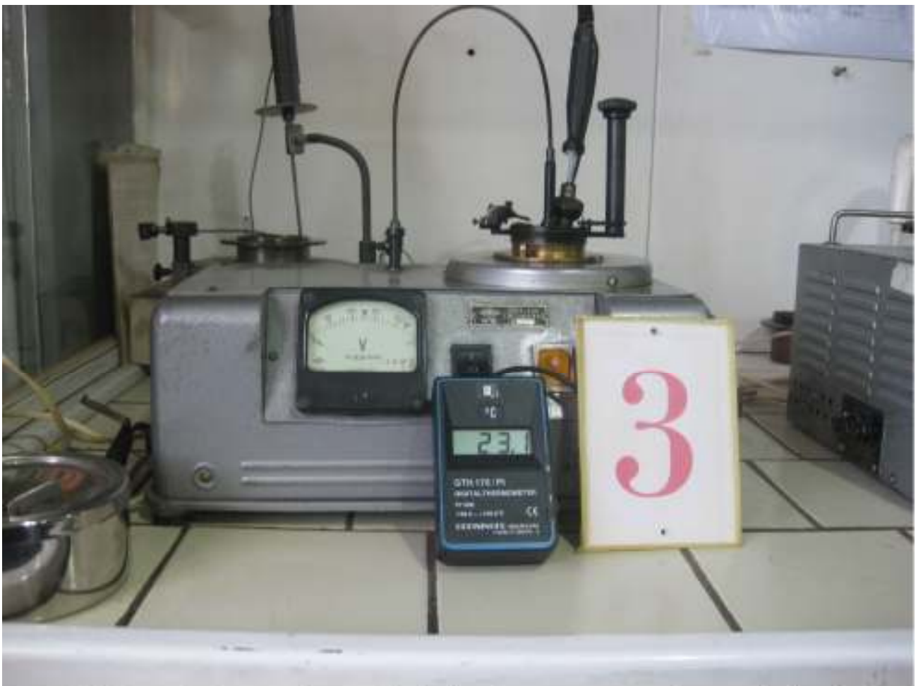
N.3 Determining transformer oils Flash point temperature by standard method
