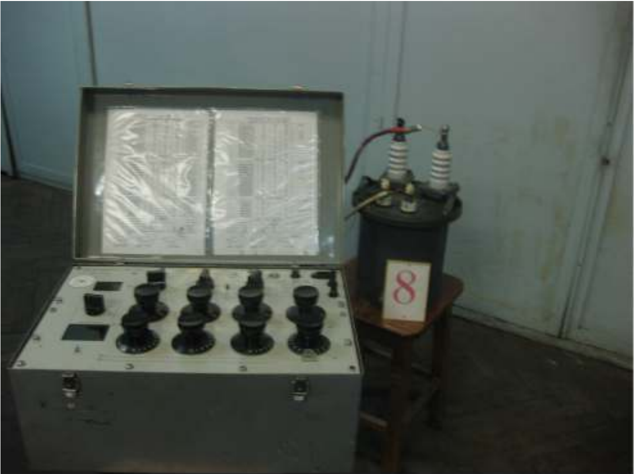
N.8 Determining high voltage transformers insulation systems dielectrical losses and capacity by standard method
