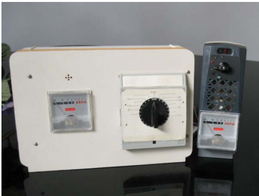
Device for measuring of compound vibration parameters. It's used for tuning various musical instruments.
