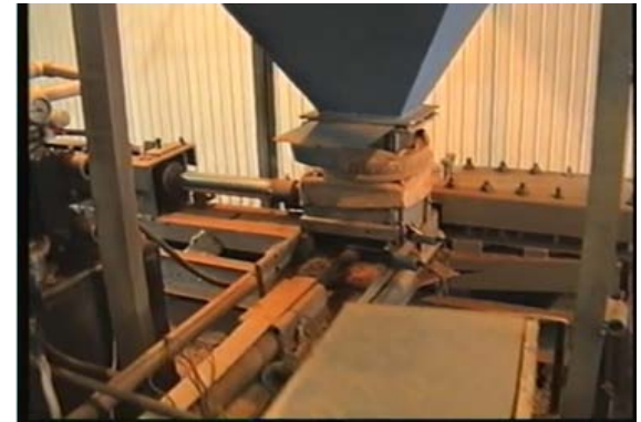
The dryer and high pressure device for production of bio-fuel briquettes.
