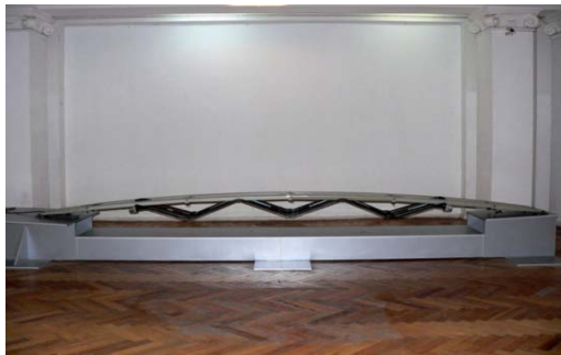
Unfolding single-span reusable bridge (L = 48 m)
