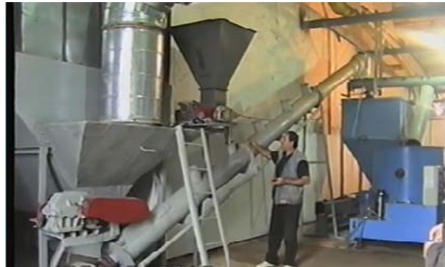
The dryer and high pressure device for production of bio-fuel briquettes.
